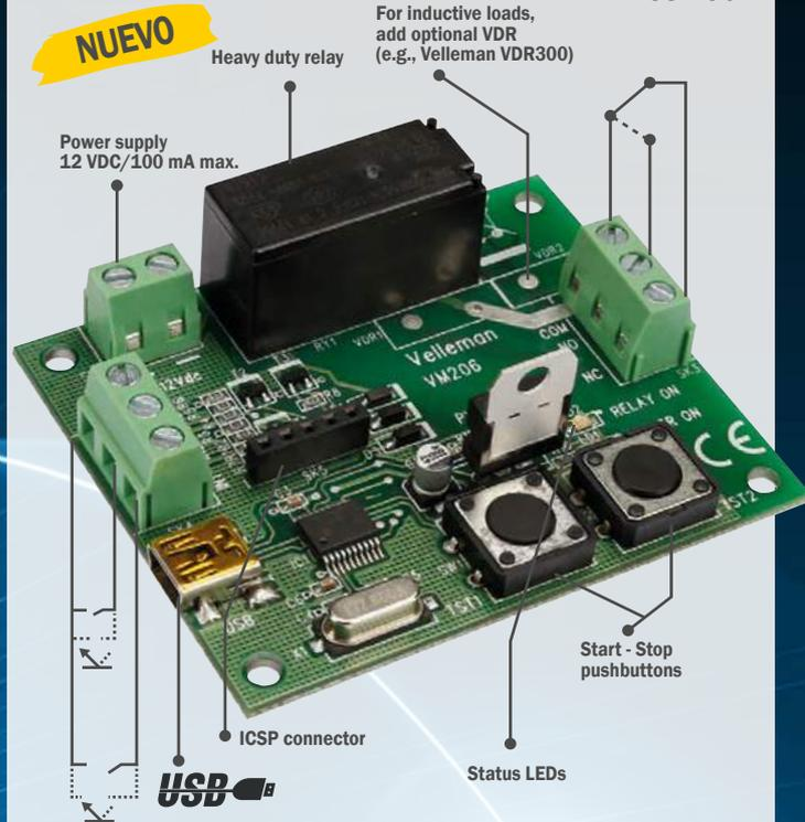
Start - Stop buffered inputs accept dry contact or open collector
